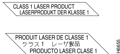
Figure 3-1 Class 1 Laser Warning Labels for Single-Mode Port
